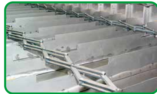
简单和复杂的剪式伸缩系统 Simple and complex shear systems at various stages.
