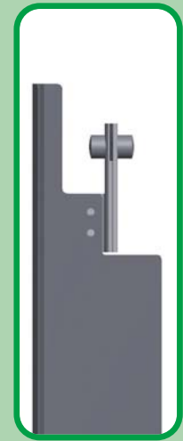
鳞甲片和钢销 Lamella with steel bolt
